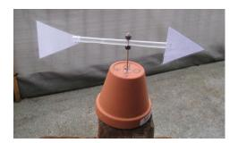
A wind direction sensor, called a wind vane or weather vane, is an indicating instrument for determining the wind direction. A movable measuring element aligns itself with the dynamic pressure of the wind.
