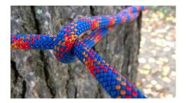
The mason's knot is suitable for attaching to trees or for hauling beams and logs with a rope. It is a tapered loop and holds only under tension. The knot is also called a carpenter's knot.
