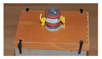
A hole the size of the lower part of the Gardena hose coupling is drilled into the top of the wooden, metal or plastic housing. The lower part of the coupling (light gray in the picture) must fit snugly into the hole without hindering the movement of the upper part. Two smaller holes are drilled to the left and right of the hole to feed the cord through.
