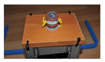
The cord is now threaded through the two smaller holes and the hose coupling module is inserted into the hole and pressed tight. It has proven useful not to glue this module so that it can always be removed for repair purposes.
