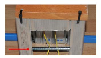
An opening is made on the side of the housing where the cord can be fed out and the bicycle pump hose fed in. In addition, a rod is inserted inside the housing to deflect the cord
