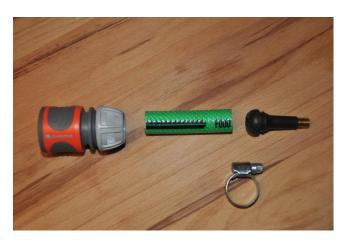
The bead of the car valve is machined until it fits snugly into the piece of garden hose. The valve is pushed so far into the hose that only the metal part is sticking out and the valve is now secured in the hose with two hose clamps. The other end of the hose is pushed into the Gardena hose coupling and secured. A cord is now attached to the neck of the hose coupling with the cable tie on the left and right. These should be several meters long.
