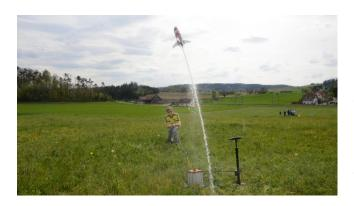
For the rocket launch, the launch pad is now placed and secured on a suitable area. The bicycle pump is connected to the car valve and the rocket is filled with water to a third of the bottle volume. The bottle is then placed on the launch pad with a quick tilting movement, if possible without losing any water.
