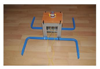
The final step is to attach brackets to the housing so that the launch pad can be fixed to the ground with tent pegs and won't tip over. I used the metal brackets from an old appliance for this. This construction won't win any beauty awards, but it does the job;)
